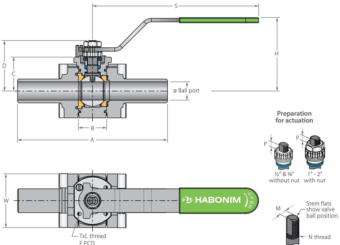
Valve Face To Face sizes are according to Habonim catalog data only, for Extended-weld/Flanged/Tri-clamp end see Face To Face sizes page.
