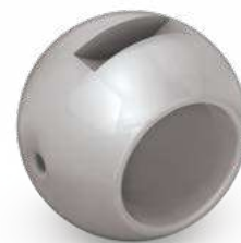
3 mm relief hole face the upstream
