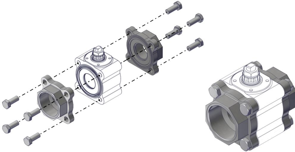
3.11. Ease back the body assembly between end connectors, taking care not to score faces or damage seals, and reinstall body bolts.
