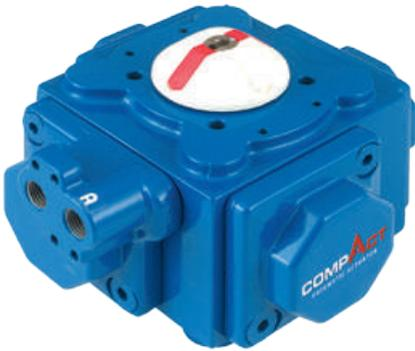
Both lines of valves were automated with the COMPACT™ 4-piston spring return pneumatic actuator. The COMPACT™ is the FASTEST, off-the-shelf, rack & pinion actuator on the market. Its unique four-piston design allows for a smaller diameter pinion, which significantly shortens piston travel and reducing response time.
