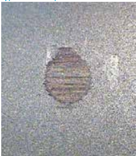
Figure 4 Typical wear dimple after 15 min
